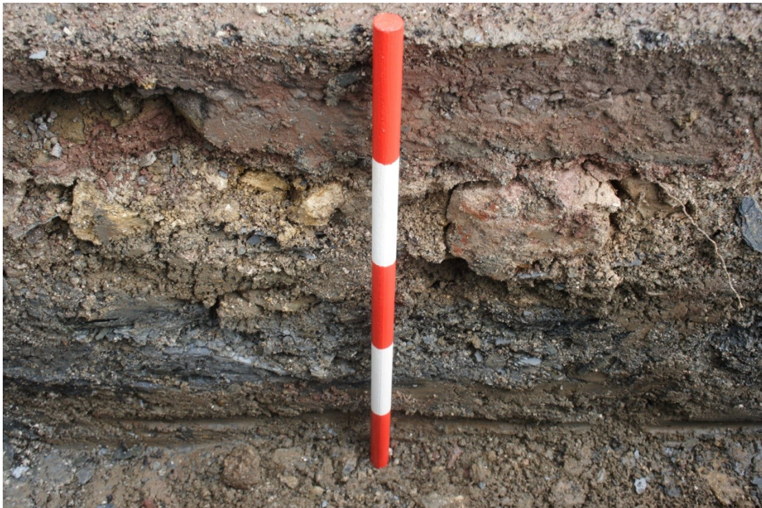
Photo 34: Different layers of sand, soil, gravel and various types of stone were found in layers making up the ground beneath the present day tarmac path
