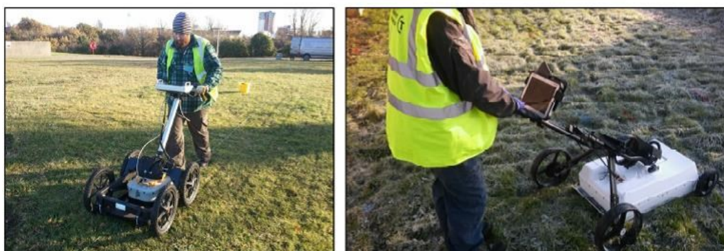
Plate 2: MALA RAMAC (left) and UTSI Groundvue 3 (right) Ground Penetrating Radar systems (library pictures)
