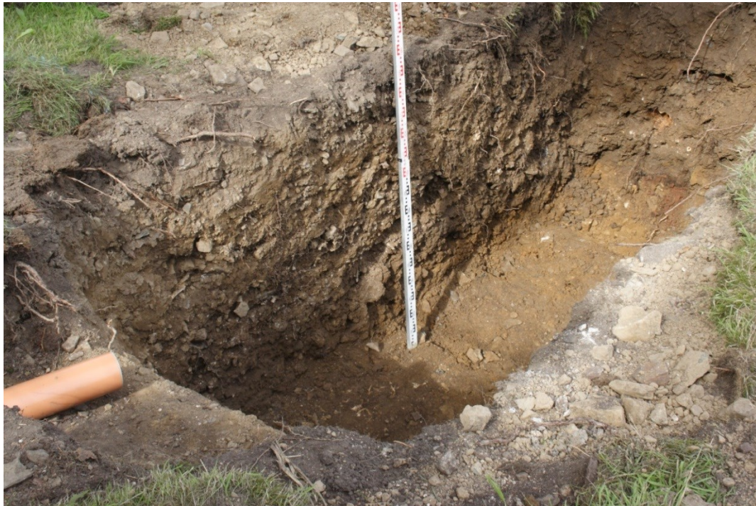
Photo 42: The north-facing section of the cess-pit trench, showing c.1m of buried building rubble beneath the topsoil, and then c.0.6m of buried topsoil with the subsoil showing at the bottom at the west end, with a 2m scale
