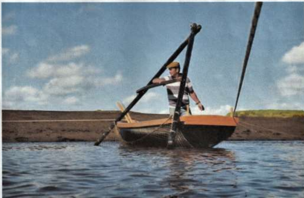
The origins of the term 'compass net' clearly demonstrated in these photos. Note the stern line of the boat taken around a thole and adjusted to set the boat at right angles to the stream.
