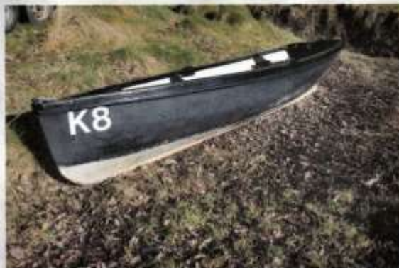
Michael Roberts' current salmon boat, a GRP hull from the Cygnus yard in Cornwall which he fitted out himself. In the traditional black Llangwm boat colour and with the K licence number on the bow, it is the nearest thing today to the old Llangwm boat.
