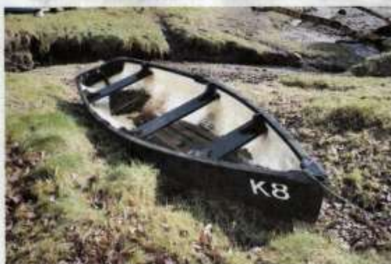
Michael Roberts' current salmon boat, a GRP hull from the Cygnus yard in Cornwall which he fitted out himself. In the traditional black Llangwm boat colour and with the K licence number on the bow, it is the nearest thing today to the old Llangwm boat.
